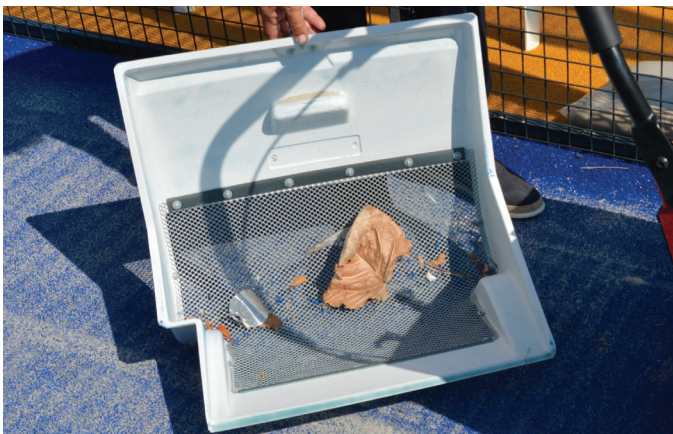
Special hopper that keeps dirt by uniformly redistributing the filling sand on padel courts.
